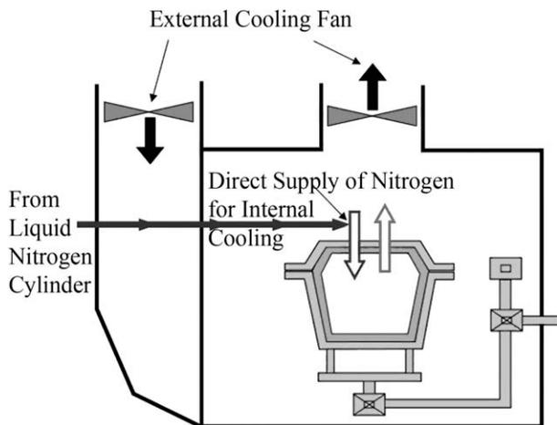
FIG. 7. Liquid nitrogen is supplied to the induction air mover and compressed air is supplied to the exhaust air mover, mold in stationary.
