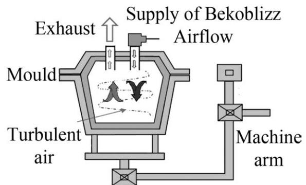
FIG. 4. Bekoblizz internal cooling apparatus.
