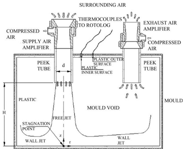
FIG. 5. Schematic diagram of the air amplifiers set up illustrating the air movement for internal cooling.
