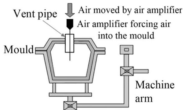
FIG. 2. Use of air mover to pump air into the mold.
