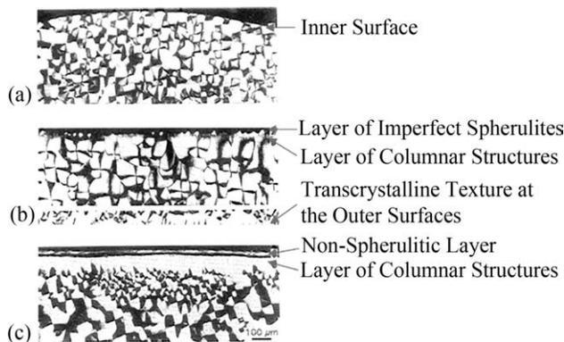
FIG. 9. Micrograph showing the morphology of polyethylene under various conditions, (a) no degradation, (b) slightly overheated, and (c) highly overheated.
