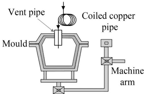
FIG. 1. Use of coiled copper pipe to bring in pressurized air into the mold.
