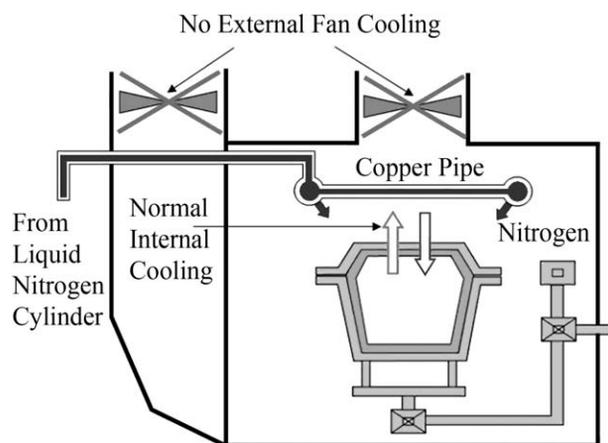
FIG. 6. Liquid nitrogen is pumped into the cooling bay and cold air is circulated into the mold via air movers.
